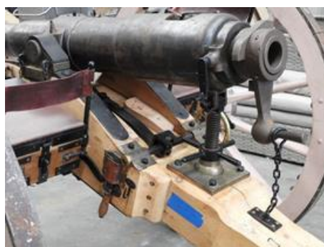
View of the breech, elevation and traversing mechanism with azimuth nut.
