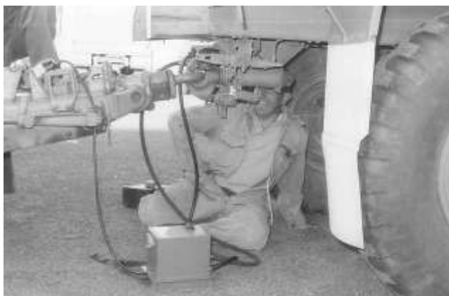
WO1 Ford attaches brake assembly to new 5-ton truck and 5.5" gun
